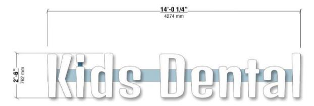
Proposed illuminated building sign with an area of 3.78m<sup>2</sup> on the third storey of the building (Sign 2).
