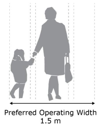
**Figure 17. Dimensions of person in mobility device**
