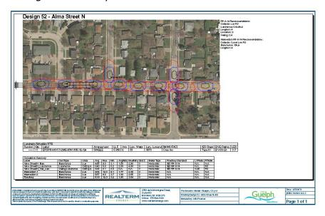
Figure 1: Sample photometric LED streetlight design
