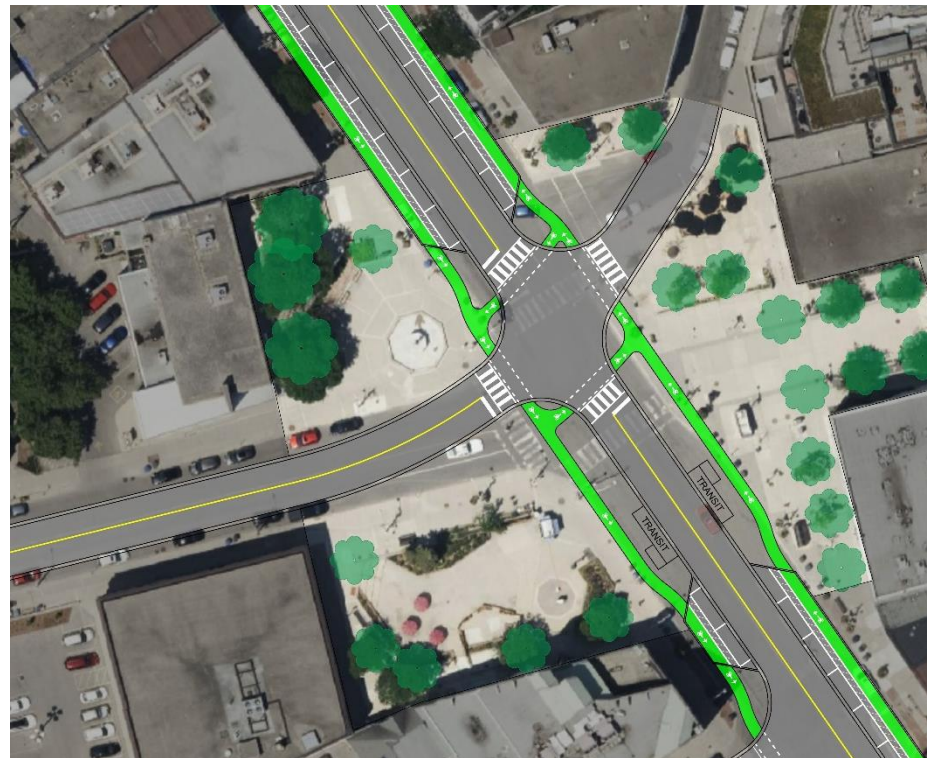
Realigned four-leg Intersection Configuration.
