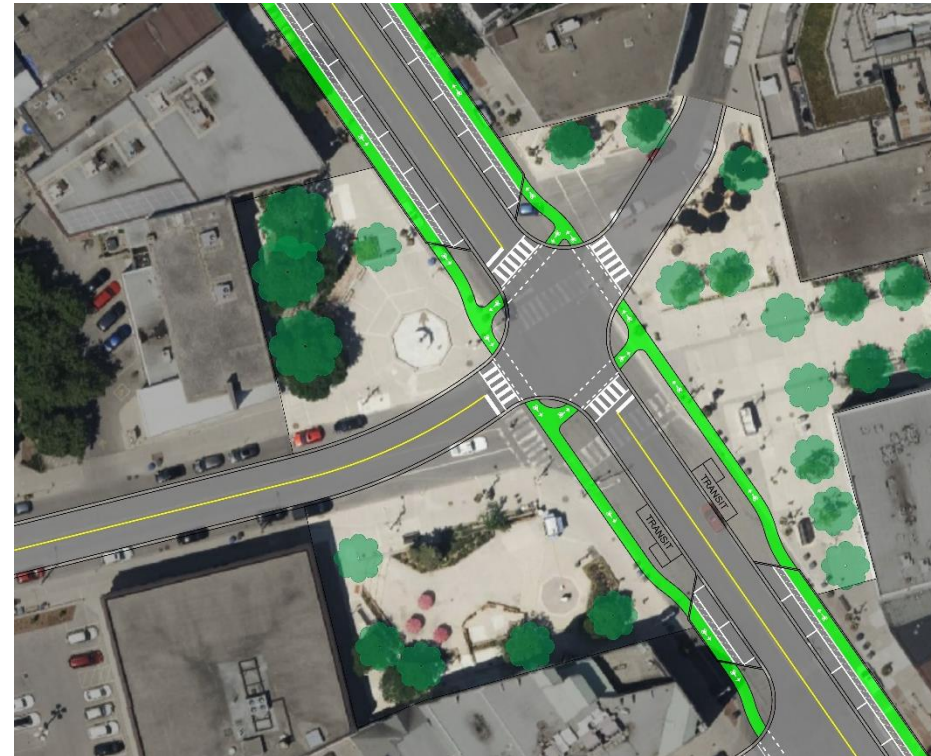
Realigned four-leg Intersection Configuration.
