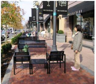
The Planting and Furnishing Zone is located between the sidewalk and the edge zone, and provides a location for site furnishings, waste storage systems and street trees, as well as a buffer between vehicles and pedestrians.
