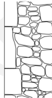
Figure 2: Ashlar Faced Rubble Wall
