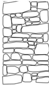
Figure 1: Typical Rubble Wall
