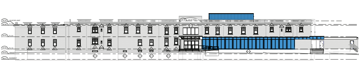
East elevation with new construction shaded blue (Cornerstone, 2024; annotated by ERA).
