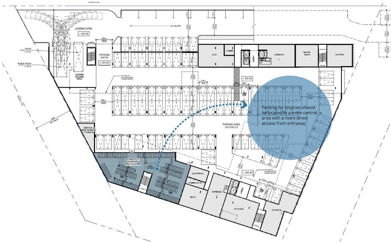
Figure 5: Bicycle parking to be relocated to the eastern side of the parking level
