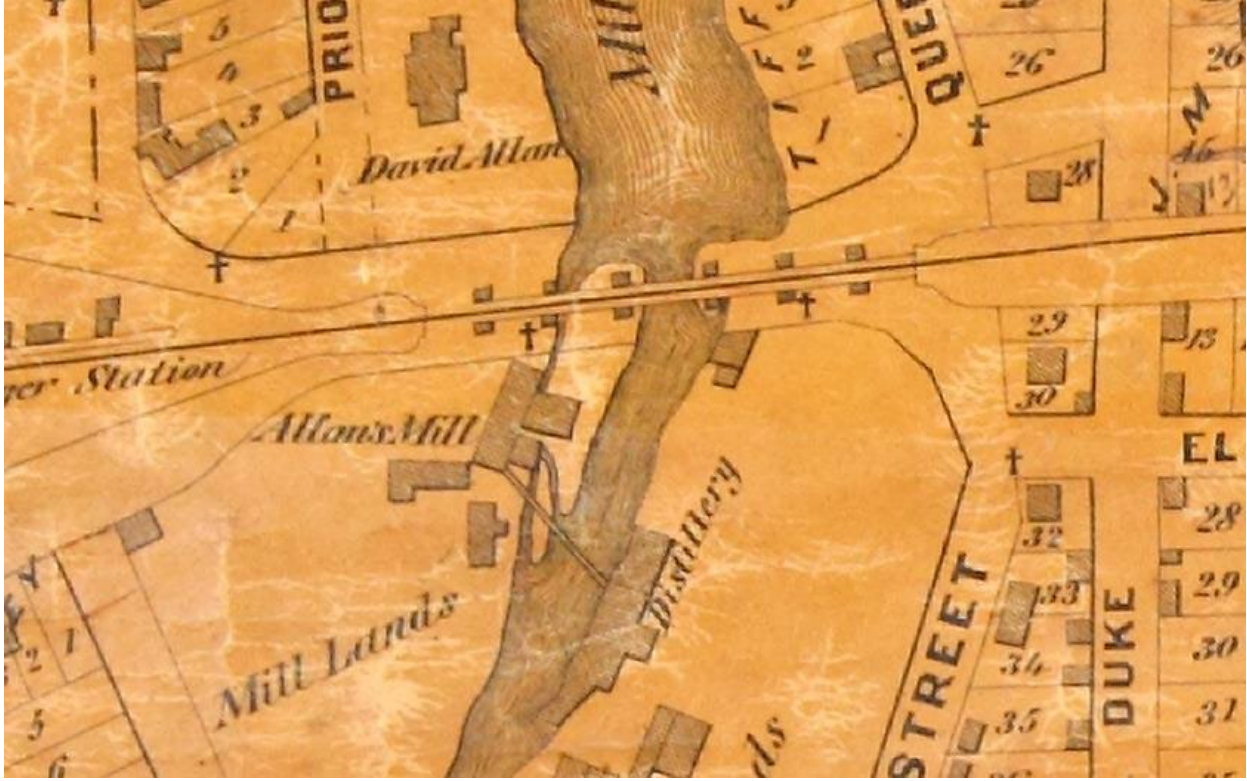
Figure 21 Detail of Cooper Map c. 1874- P. Brian Skerrett. Note the river is still narrowed between the two viaduct piers, suggesting abutments that reduce the bridge span.
