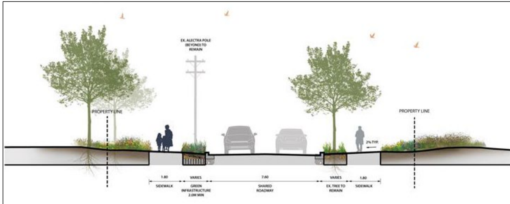
Figure 39: Typical proposed right-of-way cross section (Arup)
