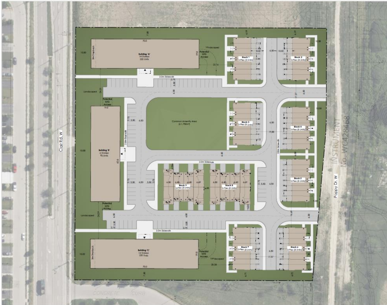
Figure 1: Proposed Conceptual Site Plan for Block 1 (lands north of the future Poppy Drive West)
