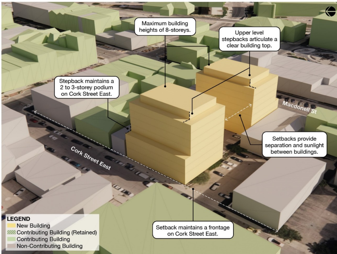
Figure 41: Illustration showing the potential redevelopment (for demonstration purposes only) of a non-contributing property that is currently vacant.
