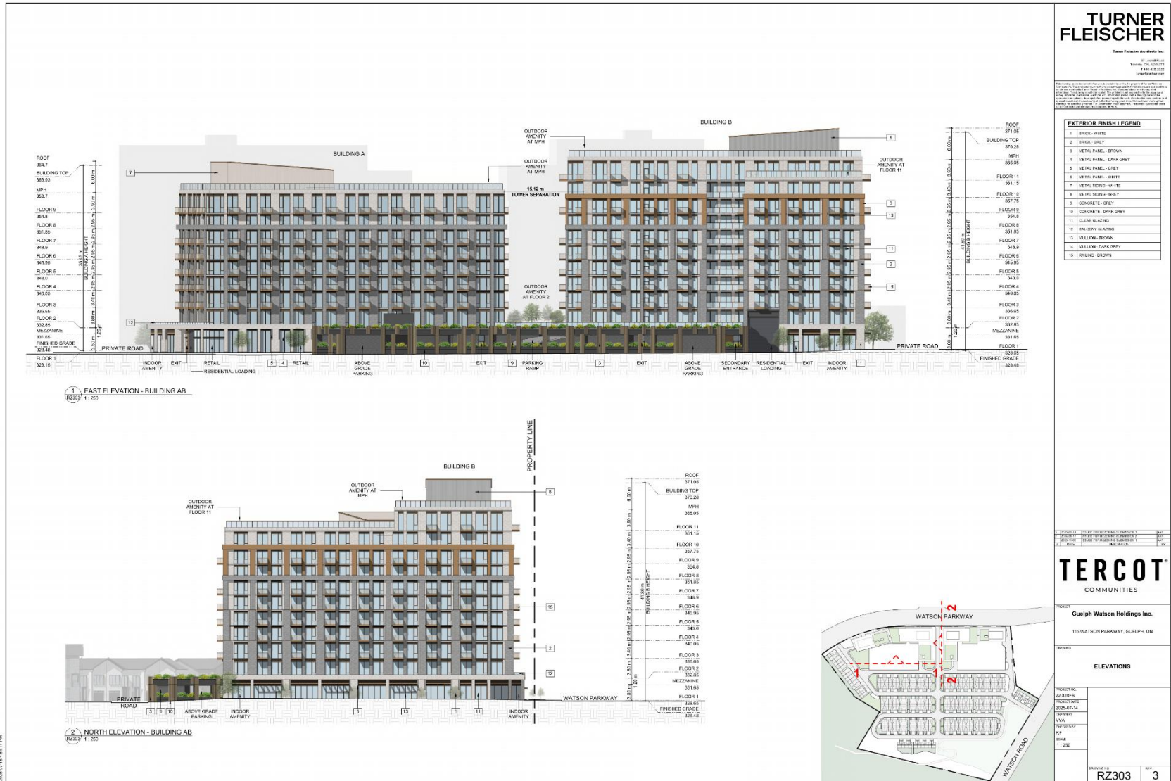
Figure 4: Proposed Building Elevations (East, North)
