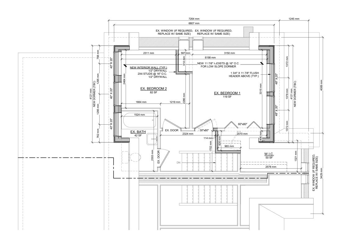
1. ALL EXISTING DIMENSIONS TO BE CONFIRMED BY THE CONTRACTOR PRIOR TO CONSTRUCTION & PRODUCTION OF PREFABRICATED PRODUCTS SUCH AS PRE-ENGINEERED WOOD TRUSSES. THE DESIGNER MUST BE NOTIFIED OF ANY MAJOR DISCREPANCIES BEFORE WORK COMMENCES
