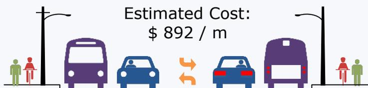
Widen Equally about Existing Centreline with Two Lanes in each Direction, a 4m Two-way left-turn lane, and Separated 3m multi-use -Paths in each Direction
