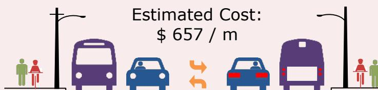
Widen on West Side with Two Lanes in each Direction, a 4m two-way left-turn lane, and Separated 3m multi-use - Paths in each Direction
